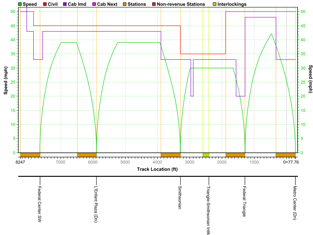
Figure 21 – Speed Profile - Final Train Fixed Block Core Segment Ideal Headway
